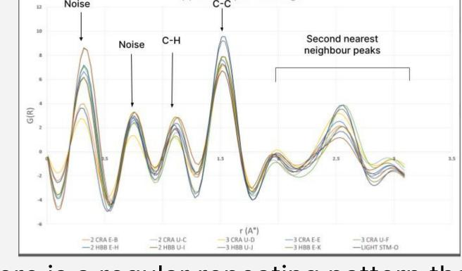
There is a regular repeating pattern that can be seen in all samples, and indicates a chemical regularity in the not-so crystalline structure of beeswax. This discovery was surprising to us.
